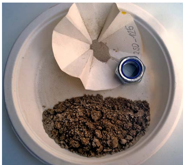
Fig. 8. Sandy clay from the Argille di Fangario formation (see text) - Sandy fraction, 250 \mu - 125 \mu interval, visual proportion of sinking and non-sinking (on filter paper) residue
