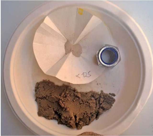
Fig. 9. Sandy clay from the Argille di Fangario formation (see text) - Sandy fraction, 125 \mu - 64 \mu interval, visual proportion of sinking and non-sinking (on filter paper) residue
