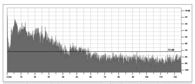
Fig. 6. Song of *Luscinia megarhynchos*. Frequency spectrum analysis of the calling song "B" (see Fig. 4) , Blackmann-Harris window type, FFT size 4096 bytes, 0-125kHz. Volume window -6dB / -103dB.
