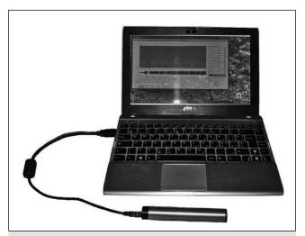
Fig. 2. Ultrasound USB recording set: Asus Eee PC 1225B notebook personal computer, USB cable and Dodotronic Ultramic 250. On the display, SeaWave software by the University of Pavia's Interdisciplinary Center for Bioacoustics.
